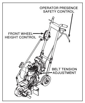
Figure 5, Edger Controls
